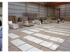
排版 Dry Lay Inspection
